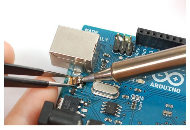
Clip the diode short and bend the leads over. Solder the side without a stripe (anode) to the old fuse pad, nearest the board edge. Solder the striped end (cathode) to the right hand leg of the regulator.
