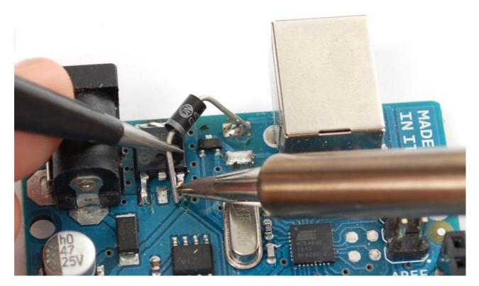
That's it! You are now 3.3V powered. This is a little lower than the power/frequency specification for the AVR chips since they ought to have about 3.6V to run 16Mhz but its *probably* not going to be an issue since AVRs can be overclocked a little.
