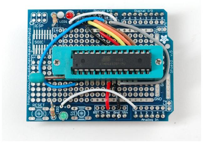
With the USB cable still plugged in (and the same Serial port selected as before) Select Tools→Burn Bootloader→w/Arduino as ISP
