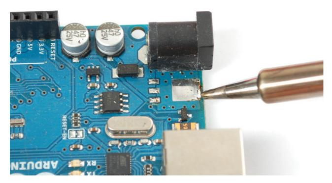
Now line up the new 3.3V regulator, and solder the tab first, use plenty of solder and be patient, the tab acts like a heat sink.
