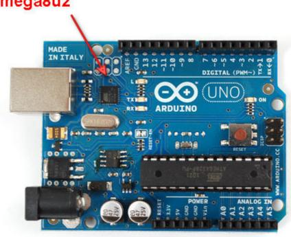
One improvement in updating the chip is that, previously, Mac users needed to install FTDI drivers. The 8u2 imitates a 'generic' CDC serial device. So now, Mac users do not have to install a driver. Windows users still need to install the .INF file but luckily there are no drivers. This means there will be fewer problems with new versions of windows. There is no way to have a serial USB device that doesn't require an INF file in windows, sadly :(
