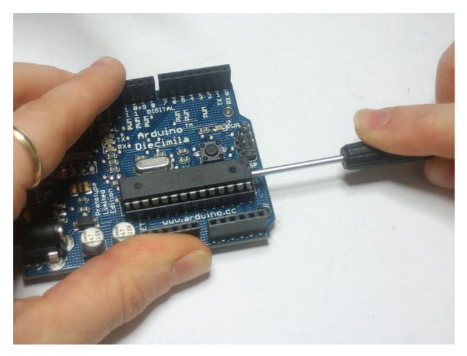
Next, prepare the new chip. The pins of ICs are a little skewed when they come from the factory, so they need to be bent in just a tiny bit, to be parallel. Grip the chip from the ends and use a table.
